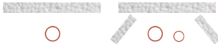
Figure 28. Thermal insulation of the pipeline using foam plates
